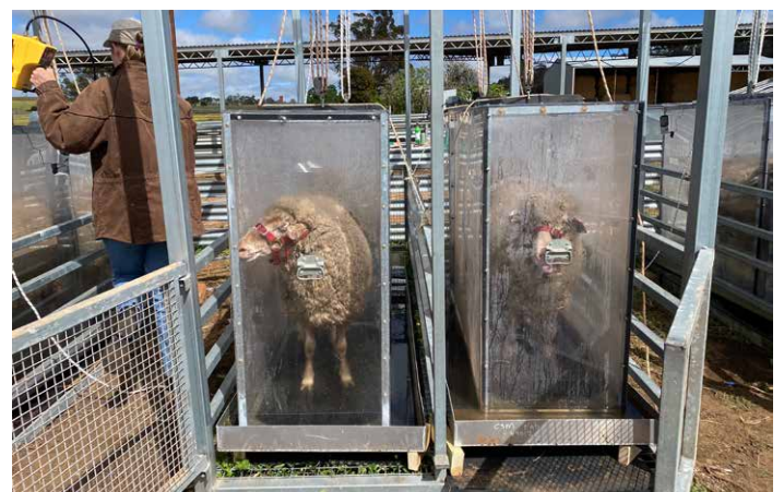
Sheep being measured for methane emissions in portable accumulation chambers (PAC)
